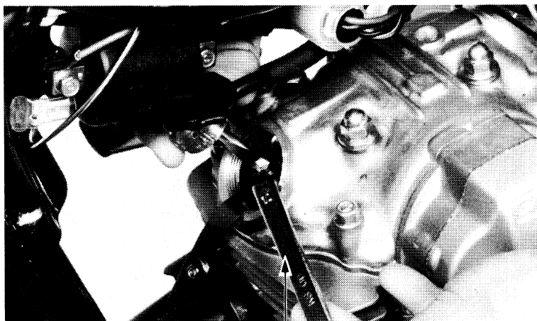
VALVE ADJUSTING WRENCH, 10 x 12 mm 07708-0030200
